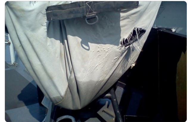
Trapped water causing corrosion and damaging the cover.
