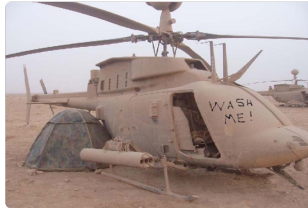
Fine sand ("moon dust") degrades components and fouls lubricants.
